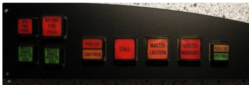
Figure A5. CRJ700 glareshield warning and caution light switches (as seen on the right side of the cockpit).
