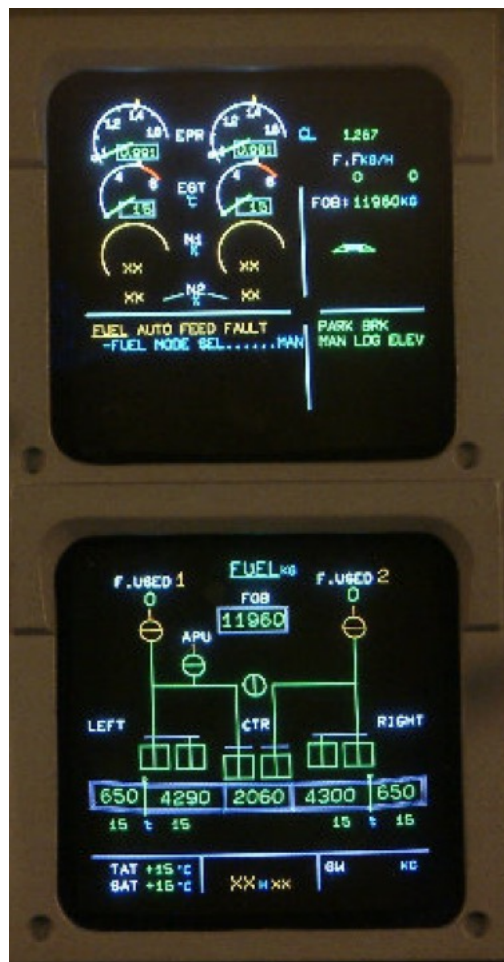
Figure A1. Airbus ECAM displays.
