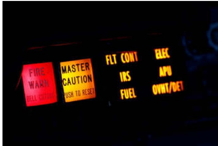
Figure A2. Boeing 737 master caution/fire warning and system annunciator lights.
