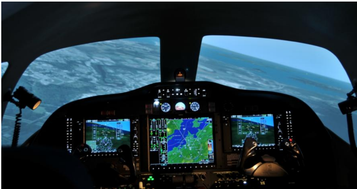
Figure 6. Simulator G1000 avionics suite and out-the-window view.
