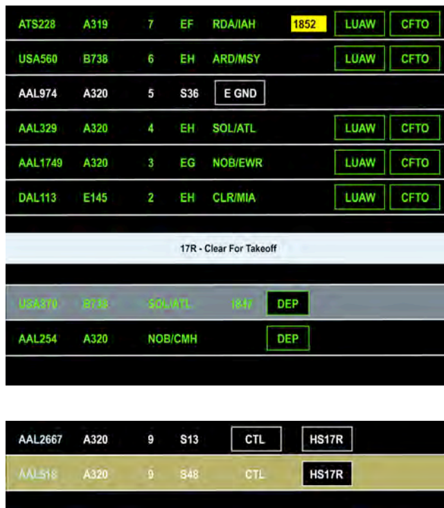
Figure 5. Local Controller SARDA departure queue (top) and runway crossing (bottom) electronic flight strip sections
