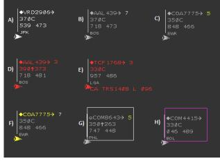
Figure 3. Expanded data tag examples.
