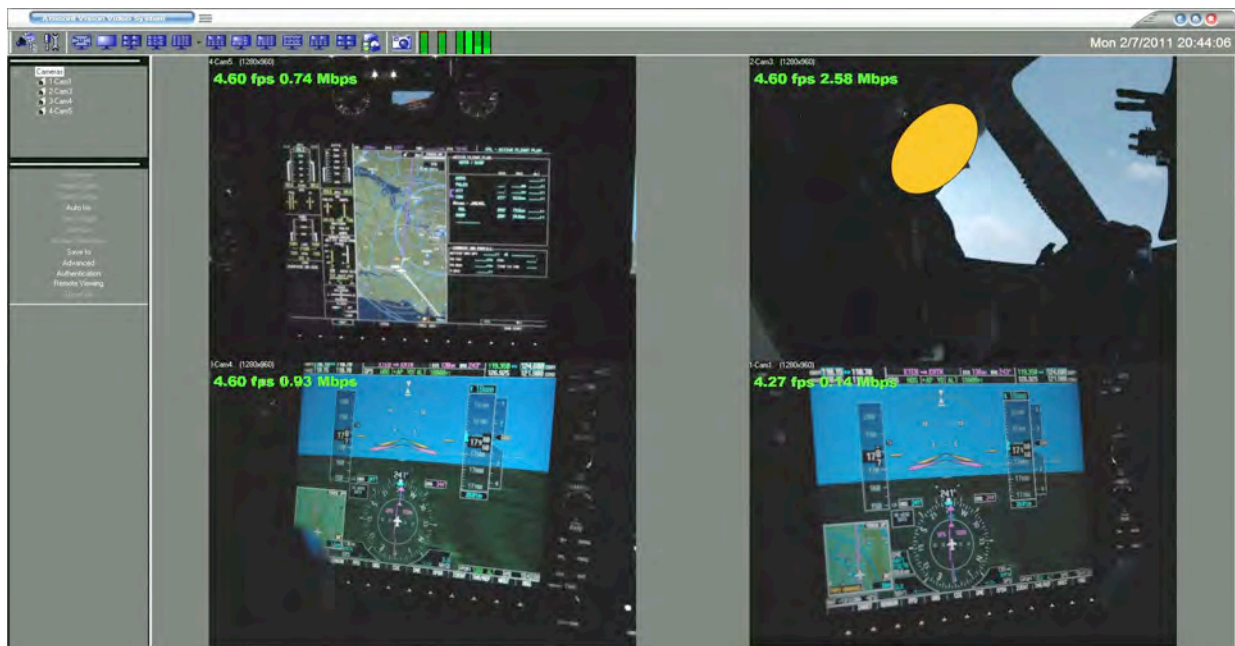
Figure 4. EMRRS output showing the four camera views. Starting from top left rotating clockwise: MFD; view of pilot; pilot's PFD; and co-pilot's PFD.
