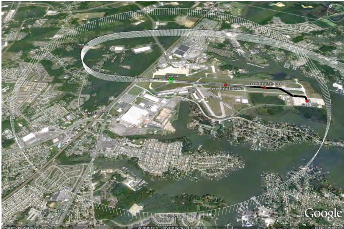
Figure 11. Plot of the 1.3 nautical mile obstacle clearance area at Martin State Runway 15.
