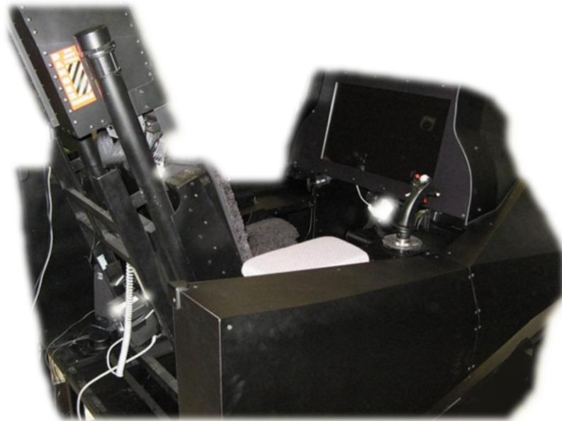
Figure 7 – OBVA Research Cockpit Configured for Fixed Wing Fighter Application
