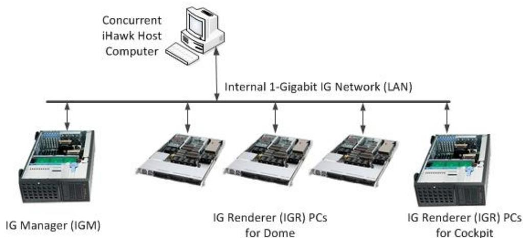
**Figure 11 – Top Level IG Architecture**
