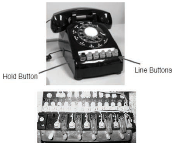
Fig. 1. Top: Western Electric Model 565 telephone. Bottom: switch assembly
