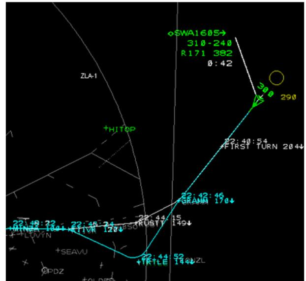
**Fig. 5** Path adjustment trial plan created by arrival planner.
