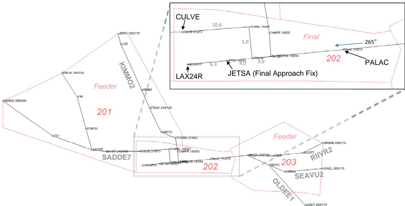
**Fig. 1** Simulation airspace and RNAV routes to LAX runway 24R.
