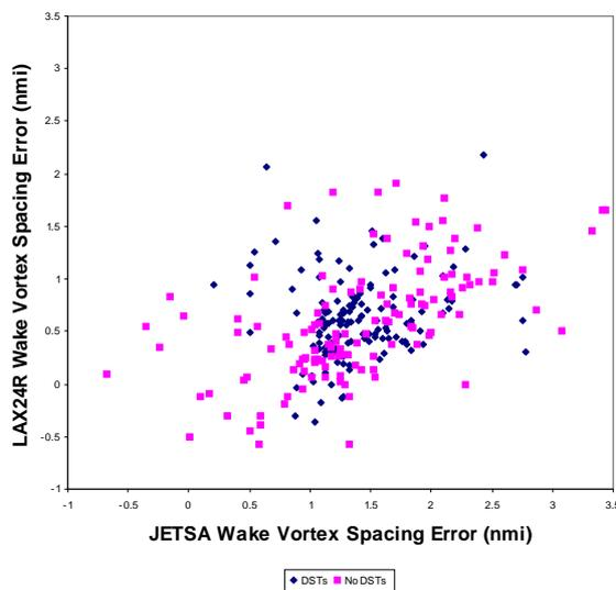
**Fig. 14** JETSA vs. LAX24R wake vortex spacing error in DST and no-DST conditions.
