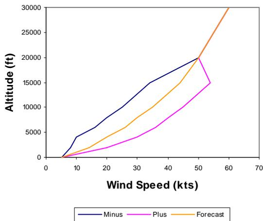
**Fig. 2** Actual winds biased from forecast winds used for trajectory predictions.
