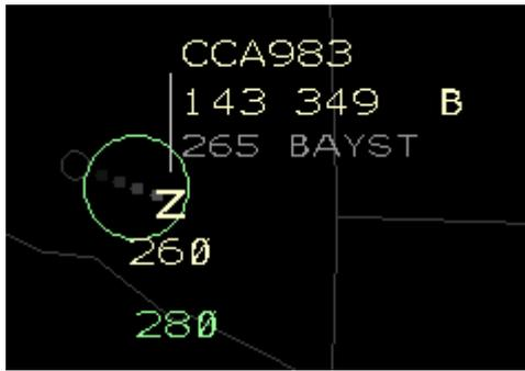
**Fig. 4** Slot marker with nominal charted profile speed (“280”) displayed in green, and speed advisory in the third line of the data block.
