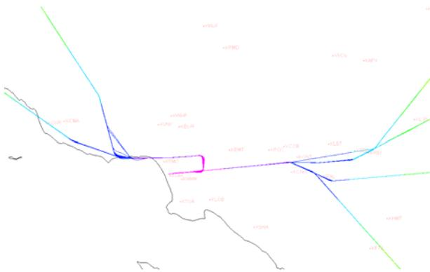
**Fig. 6** Tracks for all aircraft in nominal tools conditions (color-coding represents altitude in 5,000 ft increments).
