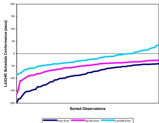
**Fig. 12** LAX24R schedule conformance data recorded in the background during no-DST conditions.
