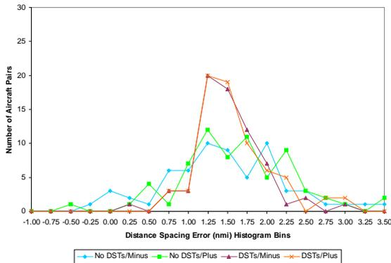
**Fig. 9** Wake vortex spacing errors measured at JETSA for the different forecast wind errors.
