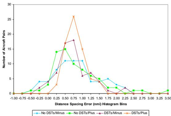
**Fig. 10** Wake vortex spacing errors measured at LAX24R for the different forecast wind errors.
