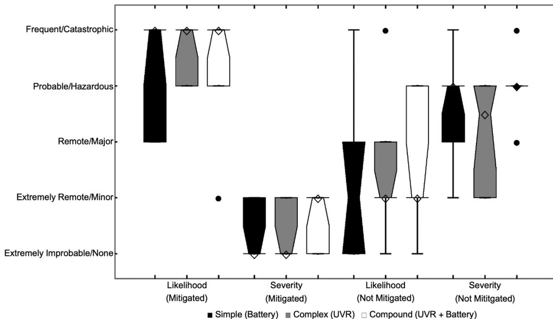
**Fig. 4** Distribution of risk rating scores, mitigated and not mitigated, by contingency. Filled circles = outliers, hollow diamonds = median values. Vertical axis labels = likelihood/severity scales, respectively.
