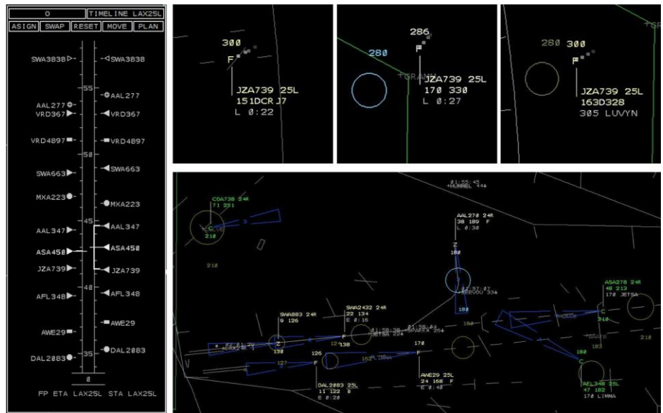
Figure 6. Clockwise from the left: (a) timeline including spacing bracket, (b) Full Data Block (FDB) with early/late indicator, (c) dwelled FDB and slot marker (d) FDB, slot marker and speed advisory (e) spacing cones and route display.
