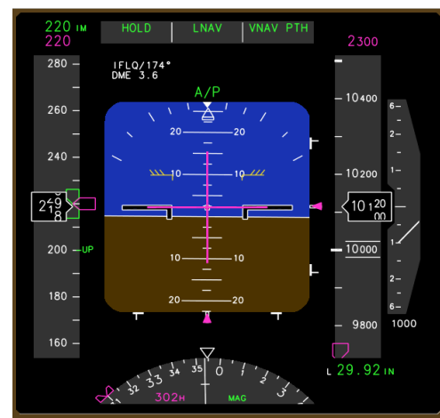
Figure 8. Primary flight display with IM speed
