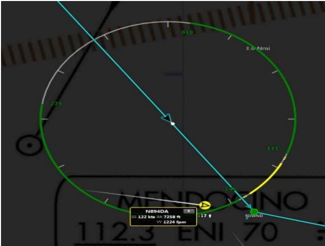
Figure 2. Lateral Omni Bands during an active Corrective DAA alert. Green bands indicate safe headings that would resolve the alert if flown.
