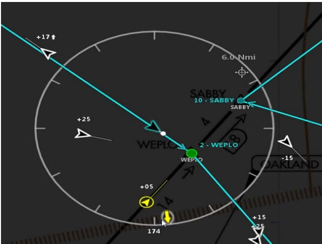
Figure 3. Lateral Vector Planning tool during a Preventive DAA alert. Solid yellow arrow indicates the specific heading selected (174°) will lead to a Corrective DAA alert if flown.
