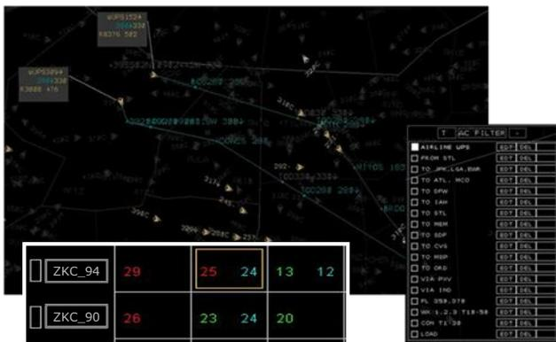
Figure 5. Multiple Aircraft Trajectory Modification Tools: Shows two aircraft being probed for combined altitude/lateral route modification.
