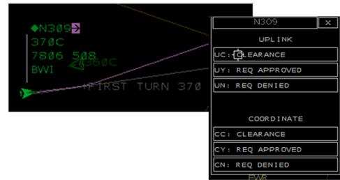
Figure 7. Trajectory change request as shown on the controller station (left); pop-up menu to uplink the trajectory clearance to the flight deck (right).
