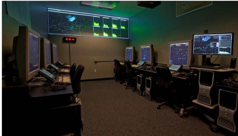
FIGURE x.2: Test Area with 4 Radar, 2 Radar Associate, and Area Supervisor Stations
