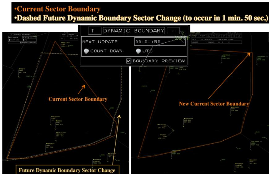
FIGURE x.3: Controller display during a boundary change
