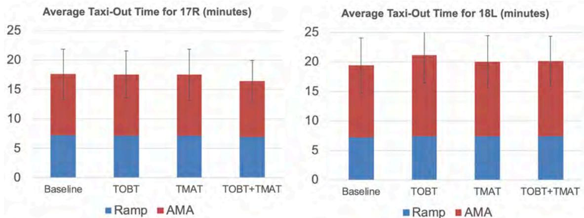
**Fig. 5 Average taxi-out time of departures from Terminals A, C, and E to Runways 17R (left) and 18L (right). Error bars are standard deviations for total taxi-out times.**
