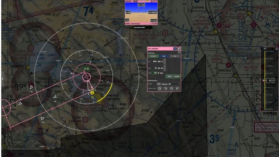
**Fig. 1** Screenshot of the VSCS TSD during a Corrective DAA alert. Intruder alert symbol and heading bands are shown near the center-left; altitude bands are depicted on the far right of the TSD.
