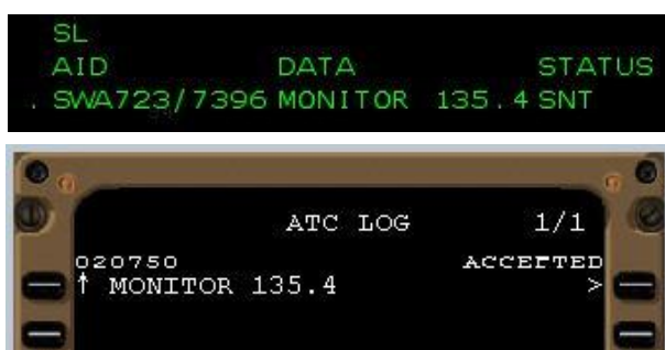
Fig. 2 View of Data Comm Transfer of Communication (TOC) message from the ATC (top) and flight deck (bottom) perspective.
