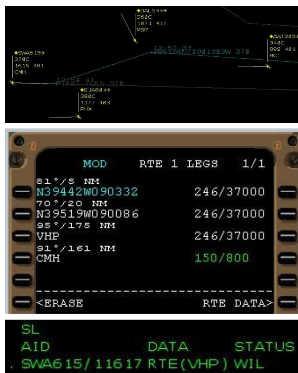
Fig. 3 A trial-plan prepared by the controller (top), then sent to the flight deck as an FMS-loadable message (middle), followed with the response message received (bottom).
