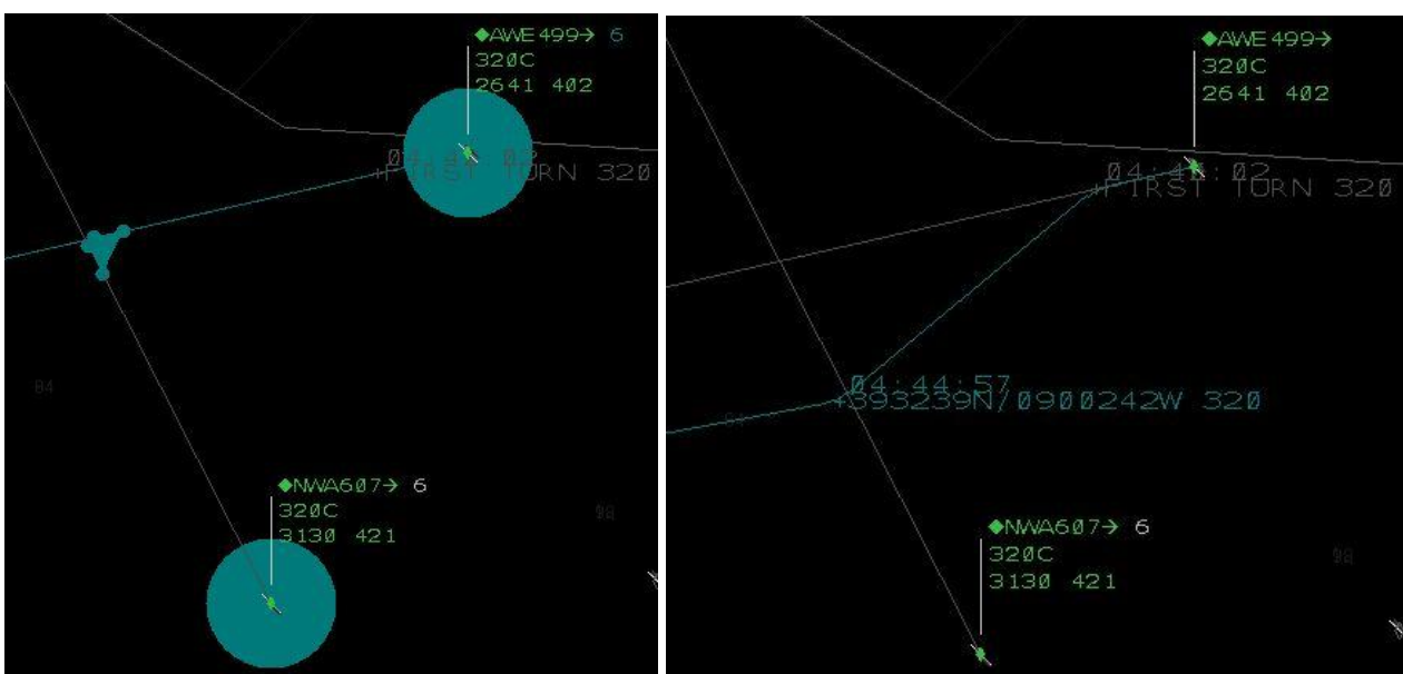
Fig. 4 The trial-planning function and conflict detection automation (left). A short visual search discovers that dragging the trial-plan to the south creates a conflict-free trajectory (right).
