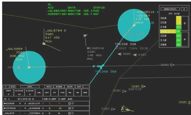
**Figure 2.** Screen image from the Minimum NextGen time-frame, showing the Data Comm status list, equipped (grey) aircraft, trial-planning capability, and conflict probe information integrated into the data blocks and altitude fly-out menu.
