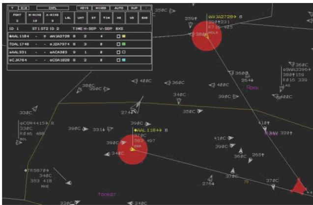
**Figure 4.** Screen image from the Maximum NextGen time-frame, showing the automation status indicators in their various colors. The small yellow box in the conflict list, signifying ‘needs controller attention,’ is coordinated with the conflicting aircraft highlighted with yellow full data blocks.
