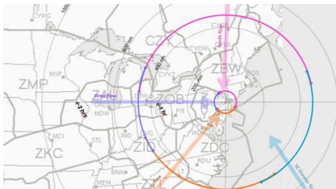
Figure 1. Schematic representation of CTOP Flow Control Arcs (FCAs): Upstream FEAs (outer arcs) and schedule to an airport (inner ring)
