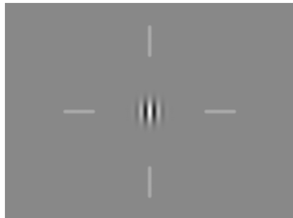
Figure 3: Sample Gabor patch image, with a contrast of one and a carrier period of 32 pixels.
