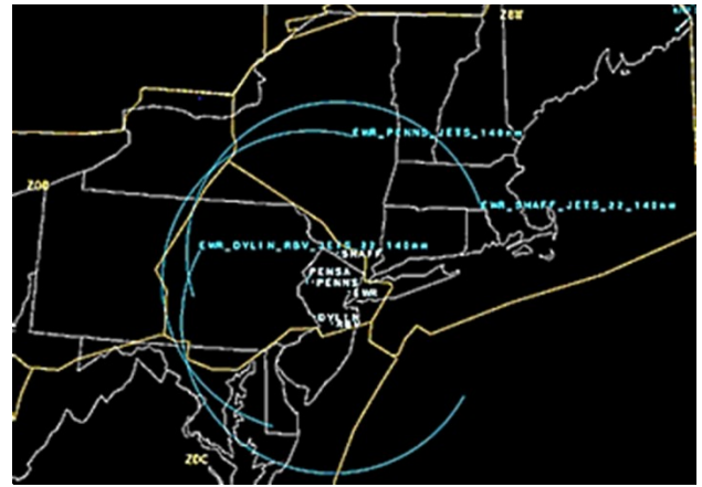
Fig. 1. Arcs are simulated TBFM MF freeze horizons for arrivals going to Newark Airport.
