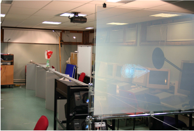
Fig. 6. The setup for the depth matching experiment showing the real object on rails (left) and the virtual object on the screen (right).
