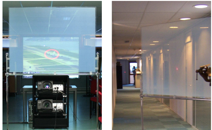
Fig. 1. The transparent projection screen demonstrating a simple overlay (left) and during the refraction experiment (right).
