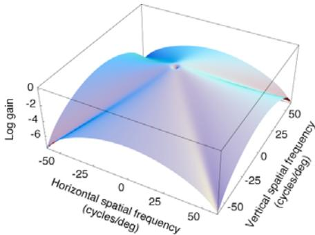
**Figure 2. Contrast sensitivity function of the spatial standard observer.**
