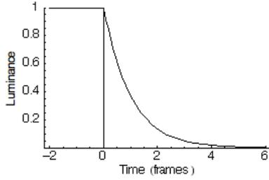
**Figure 5. An exponential transition function with a time constant of  $\tau = 1$  frame.**
