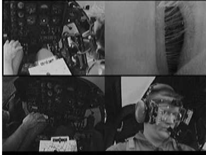
Figure 4. Sample recorded frame showing quad tiling of images from the four cameras. Upper left: fixed camera looking down and to the right over the subject pilot's left shoulder; the right hand and knee of the safety pilot is seen at the left edge. Upper right: subject pilot's right eye (rotated due to camera mounting). Lower left: image from forward-looking head-mounted scene camera, providing the "subject's eye view." Lower right: view from fixed camera on the instrument panel looking up at the subject pilot's face.
