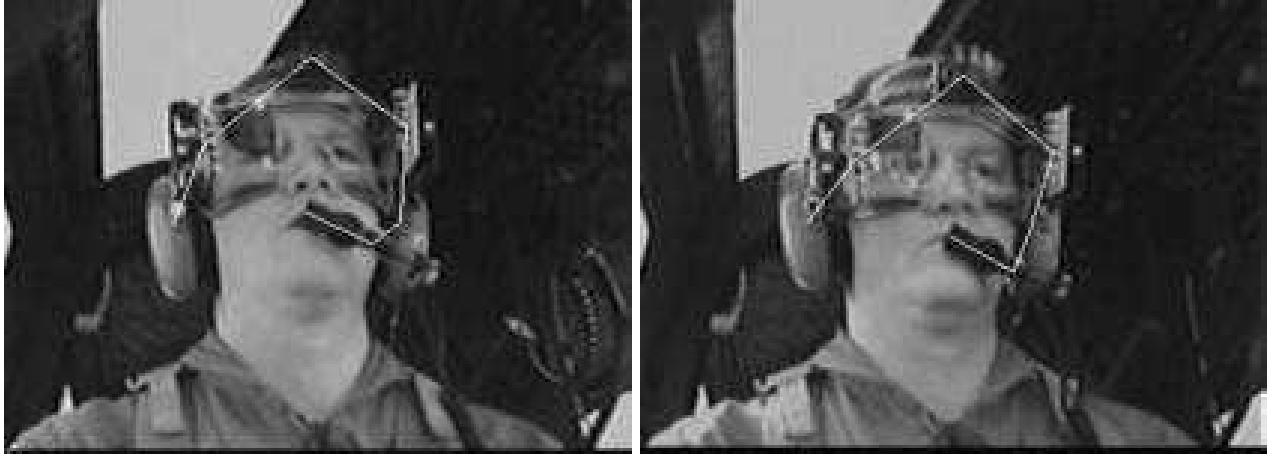
Figure 6. Image from “face-cam” with superimposed rendering of rigid 3-D space curve linking tracked features.
